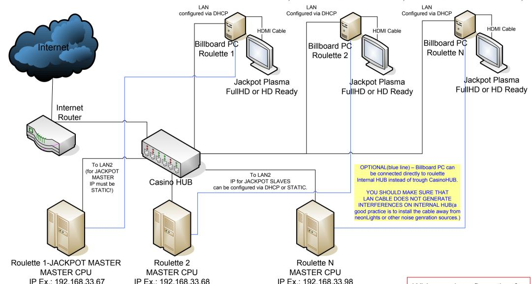
Roulette 1 will be confugured as JACKPOT MASTE. No configuration is needed – each roulettee is JACKPOT MASTER is by default. Roulette(s) 2 until N have to be confugured as JACKPOT SLAVE(s). In file /RouletteMaster/RouletteTunnel/RepetitorTunnel.conf the IP of JACKPOT MASTER has to be entered under serverhost keyword(ex.: serverhost 192.168.33.67). And in Pope->GAME\_CONFIGURATION string value for parameter JACKPOT\_DB\_SRV has to be set to '127.0.0.1:3591'
