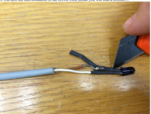
4. Unsolder the resistor from LED and brown wire as shown on picutre
