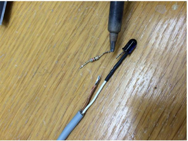
5. Instead of the resistor connect the brown wire with a piece of wire as on picture. Add also a piece of insulation...
