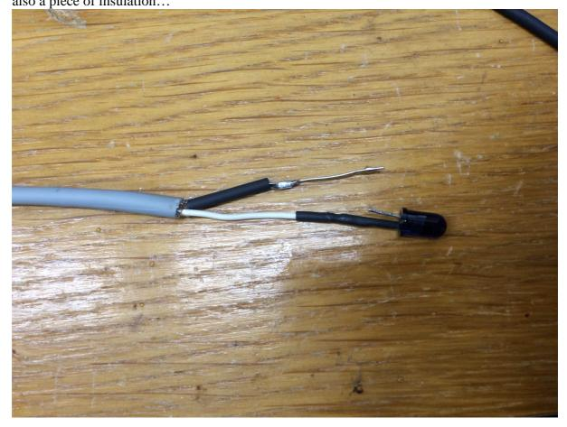
6. When you finish the LED should look like on the final picture, without the resistor. Mount the modified led back on the EJECT BOX and connect it again to 1.3 on WIN1-EJECT sensor.
